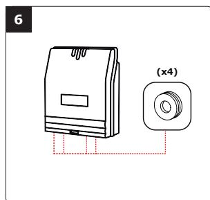
Insert the cable in the remote electronic and wire the cable to the terminals. Don't forget to install the varistor on the lock (refer to page 3, Notes and Recommendations').
