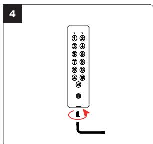
Fasten the PROFIL100EC keypad to the back plate by using the supplied (M5x8) Diax® screw and T20 Diax® spanner hardware.
