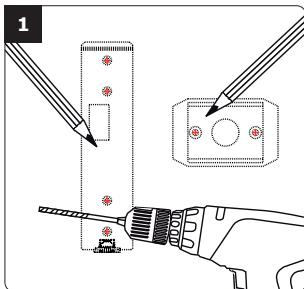
Verify the distance between the PROFIL100EC keypad and its remote electronic (refer to page 3, Notes and Recommendations). Place the back plate of the PROFIL100EC on the wall and the bracket of the remote electronic then mark with a pen the hole location then drill the 2 mounting holes (5mm drill bit Ø and 35mm hole depth) and the hole wiring access.
